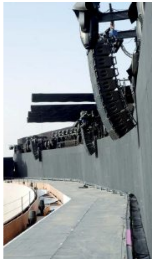
Three arrays of eight Kara in a left-centre-right configuration were used for the performance
