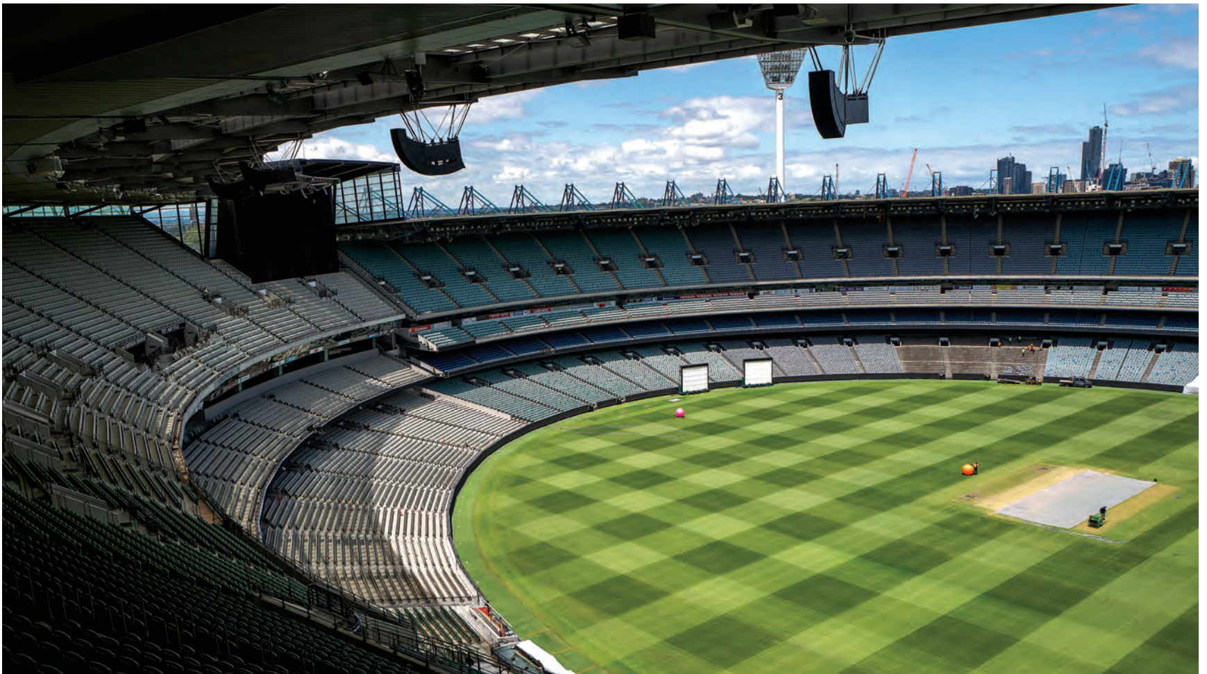
d&b V- and Y-Series modules are affixed to the bowl with custom frames
